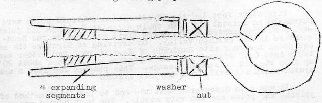
This belay will be strong enough for any normal use. One of these was tested to destruction and withstood 11 cwt. at right angles to the axis of the bolt before fracture. The bolt should withstand a larger load in an axial direction. The makers guarantee them to withstand 1000 lbs in any direction without breaking.
