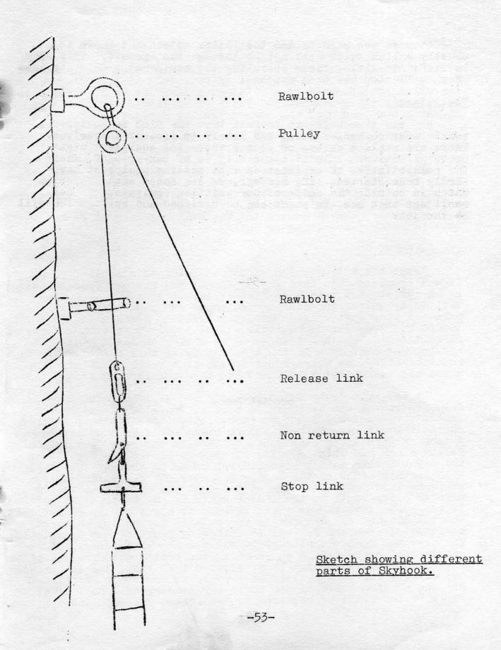
Between the skyhook and the ladder attachment there is usually a link which will not go through the eyebolt. This stop is useful in giving those operating the equipment a definite idea of when the top has been reached.
