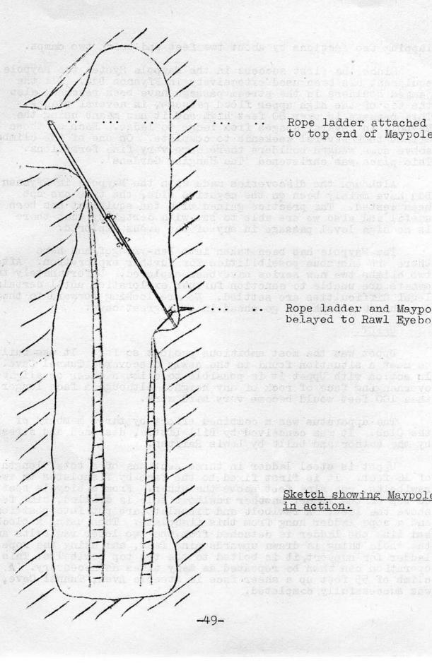
.. .. Rope ladder attached to top end of Maypole.
