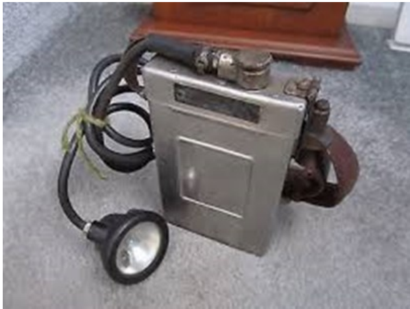
A 'NiFe' miner's lamp of the sort Dai confirms he probably used. These did have a habit of leaking caustic alkaline electrolyte (not acid as Dai suggests).
