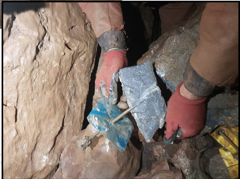
Figure 6, right. Firing pin embedded in the rock.
