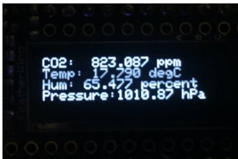
Figure 3: Screen grab of the OLED display
